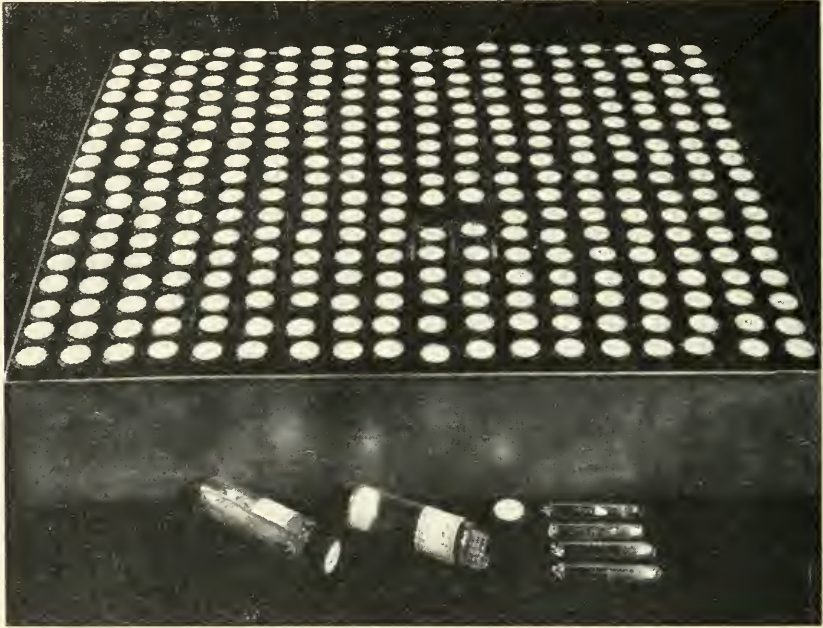
FIG. 22. Storage of tyopillized cultures, showing the limited space required. A metal box 12\frac{1}{2} inches by 14\frac{1}{2} inches will accommodate 306 vials, each containing four desiccated preparations as shown.
