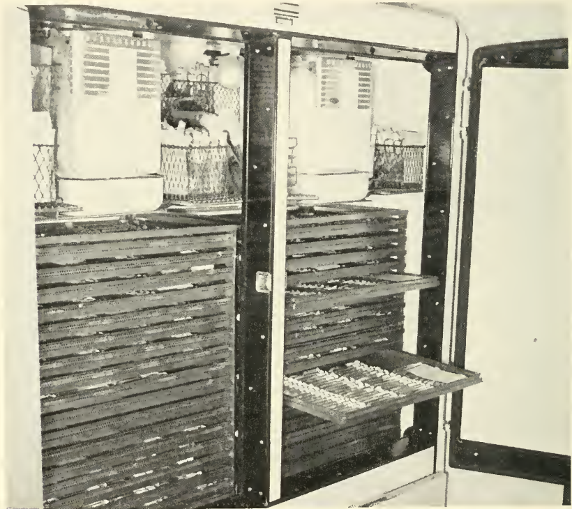
FIG. 20. Refrigerator adapted for storage of stock cultures of Penicillia and other molds. The flat sliding trays are fashioned of perforated brass sheeting to permit free circulation of air.
